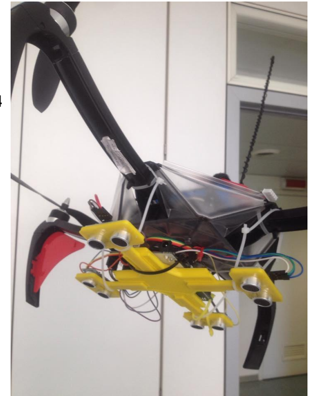
Ultrasonic Sensor SR-04
